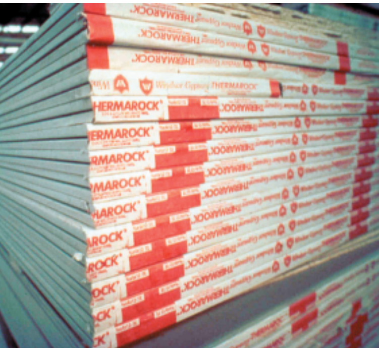
Above: This countertop manufacturer uses a recycled mixture of glass and fly ash to create durable, inert materials including counters, flooring, and benches. Left: Scrubber materials can be made into synthetic gypsum for wallboard.
