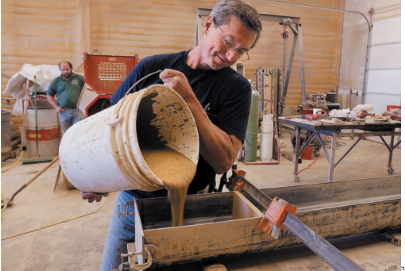
Above: This countertop manufacturer uses a recycled mixture of glass and fly ash to create durable, inert materials including counters, flooring, and benches. Left: Scrubber materials can be made into synthetic gypsum for wallboard.
